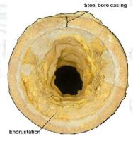
Scale Build Up Iron scale can build up over time to severely restrict the flow of water from the bore.
